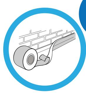
The flashing tape is laminated with either a lead or aluminium effect material
