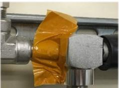
To see contrast of the color-changed area versus the non-changed area, apply tape around an area larger than the expected leak location. If the color of the whole tape is changed, it may be difficult to recognize the leak point. It is better to apply the tape over a wider area.
